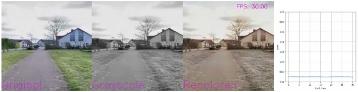
Figure 1: OpenCV window on the Jetson Nano displaying the original, grey, colorized camera stream and corresponding loss between original and colorized image.
